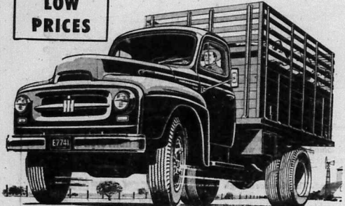
International Model R-160 with combination form body, R-160 Series, GVW ratings, 14,000 to 17,000 lbs.
