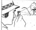
A simple locator that uses a triangulation tool to help a fisherman return to a particular location or aid campers in returning to a specific spot on land.
