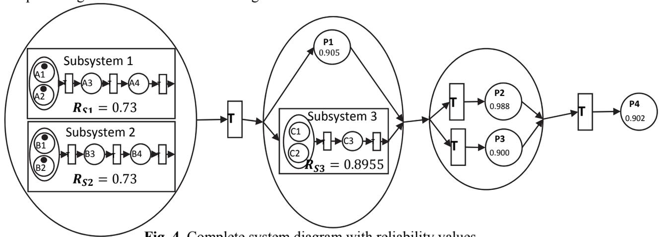
**Fig. 4.** Complete system diagram with reliability values
