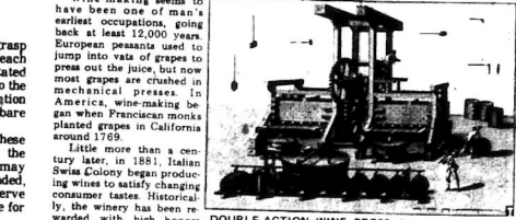
DOUBLE ACTION WINE PRESS - invented by mechanic named Abbe Legros in the 18th century, it can be worked by one man, crushing grapes and siphoning juice into barrels.
