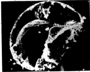
LUNAR SPECIMEN The U.S. Geological Survey is still hard at work analyzing assorted lunar specimens brought back to earth by U.S. astronauts. One of the more unusual is the one shown in this micrograph, taken on a scanning electron microscope equipped with a x-ray analyzer. The sphere portion measures about 26 micrometers (about 1/1000th of an inch), and consists of meteoritic iron and iron sulfide imbedded in a matrix of lunar glass.
