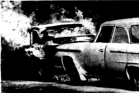
HOT CAR . . . This car exploded into billowing flames outside Frankfort recently when hit from behind at only 5 mph. The burning car carried a small can of gasoline in the trunk. No one was killed because the cars were empty. The explosion was a demonstration set up by state Fire Marshal Warren Southworth to show the dangers of carrying spare gas cans in car trunks. "The plastic gas cans many are putting in their trunks," Southworth said "are illegal in Kentucky and have been for years. Moreover, it's just very, very dangerous."
