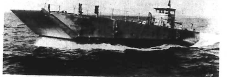
THE ARMY'S NAVY—A LCM-8 landing craft gets underway during initial production testing. The aluminum-hulled craft built by the Marinette Marine Corporation, is being evaluated by the U.S. Army General Equipment Test Activity, Ft. Lee, Va. (U.S. Army Photo by Sp4 P.J. Tocco)
