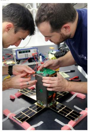
Morehead State University and its partnersreport contact has been established with the Cosmic X-Ray Background Nanosatellite (CXBN). The Cosmic X-Ray Background Nanosatellite (CXBN)-- codenamed "Unbridled Spirit" is a loaf of bread sized, five-pound nanosatellite designed to be one of the first "cubesats" to undertake a significant science mission.
