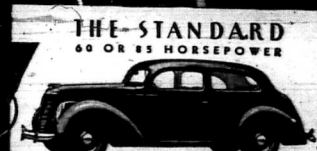
THE STANDARD 60 OR 85 HORSEPOWER STANDARD FORD V-8... 112" wheelbase; 60 or 85 horsepower engine; Improved Emergency Safety Brakes; Center-Pole Ride; All-steel body; Broadcloth or Mohlar upholstery; Mohlar extra in '60'; Mohlar-optional in '85'; One tail light, sun visor; Twin horns; 3 body types; 5 colors.
