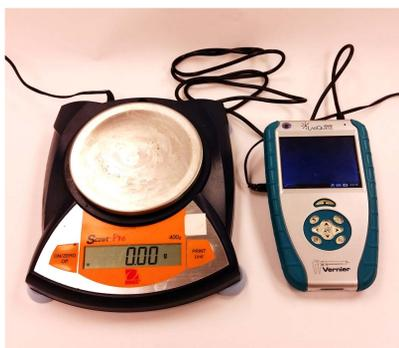
Figure 4. Talking Labquest and balance for determining mass audibly.
