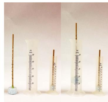
Figure 5. Graduated cylinders with floats for determining volumes of non-volatile solvents.
