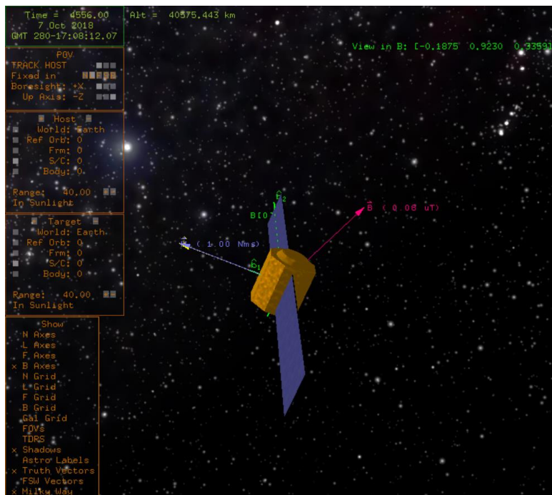
Lunar IceCube stabilized and aligned with the sun vector
